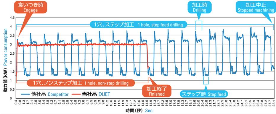
他社品は1穴目で切りくずが絡まり加工不可。DIJETは切削力も低く安定加工かつ穴精度も良好。DIJET reduced power consumption and achieved stable machining & good hole accuracy. Competitor stopped machining at the first hole due to clogging with chips.
